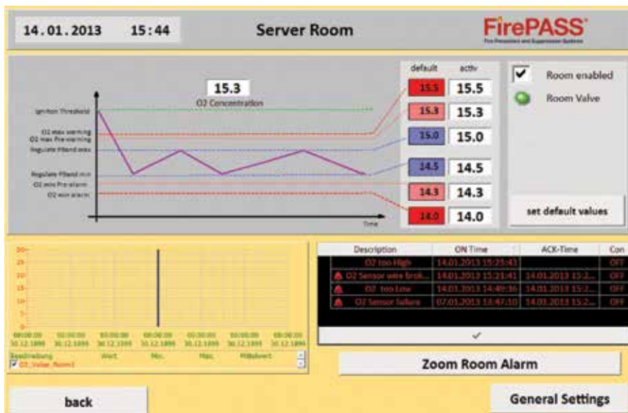
Example: The “room info screen” shows all relevant system parameters including actual and past oxygen values.
